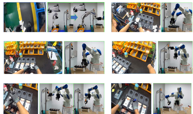
Fig. 18. Automatically generated robot unit tasks based on the human assembly script for power breaker assembly, including picking parts, assembling parts, grasping tools, bolting, and inspection.
