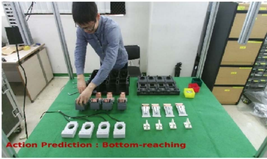
Fig. 5. Example of action prediction for a single frame, where the prediction result is “reaching toward the bottom part of the object.”
