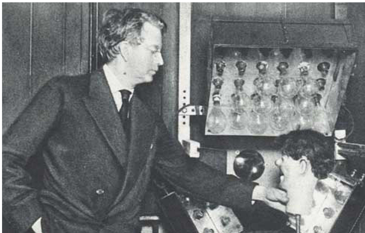
Fig. 2. Baird with his transmitter believed to be used for the first demonstration of television in 1926 [14]. One of the 30 lenses can be seen to the left of the dummy's head mounted in a plywood, 1.5-m diameter scanning disk [4, p. 55].
