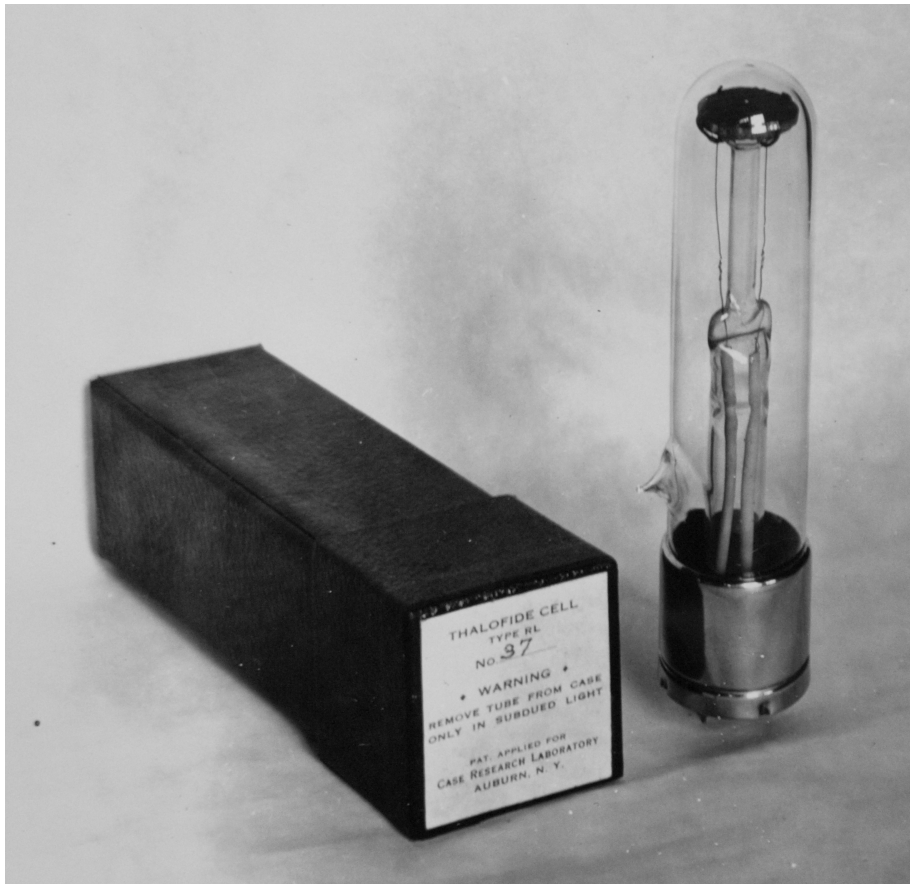
Fig. 3. Thalofide cell packaging with cell (10 cm in height approx.) on the right. Courtesy of the Cayuga Museum and Case Research Lab.
