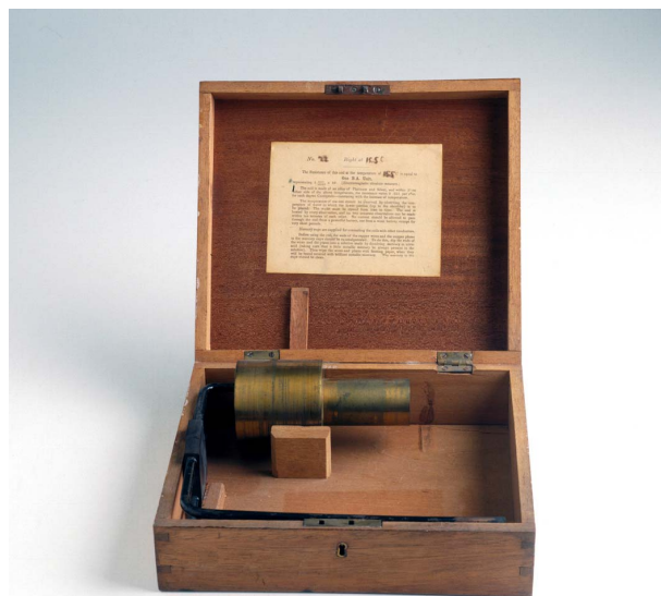
Fig. 5. BA Standard Resistor as first purchased by Michael Faraday in 1865, copyright London Science Museum, Science and Society Picture Library, rights reserved.
