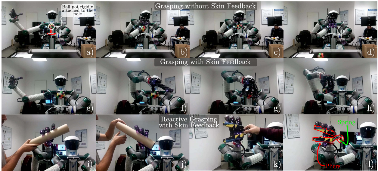
Fig. 13. Reactive grasping using multimodal robot skin information. (a)–(d) Global grasping using simple primitives. (e)–(h) Enhanced reactive grasping using robot skin. (i)–(l) Reactive grasping for multiple objects and applying different force profiles.
