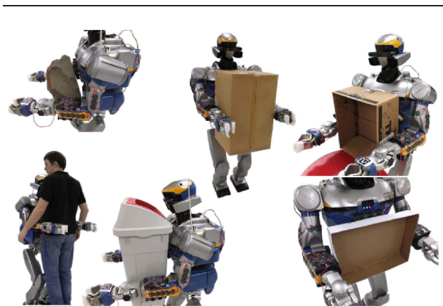
Fig. 14. Humanoid robot safely holding objects using the information from the robot skin and applying a sensory-motor map.
