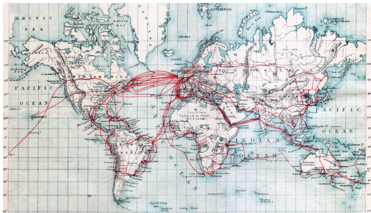
Fig. 2. Cable map of the world, 1901, from W. Clauson-Thune, A.B.C. Telegraphic Code , 5th ed. London, U.K.: Eden Fisher & Co., 1901, courtesy of Bill Burns. The dashed lines in the Pacific represent cables then in the planning stages; the one from Canada to Australia and New Zealand was completed in 1902, while the one from California to Hawaii was laid at the end of that year and extended to the Philippines in 1903.
