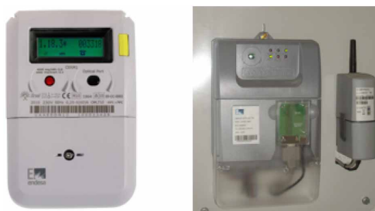
Fig. 24. Smart meter and concentrator installed in Smartcity Málaga (courtesy of Endesa).
