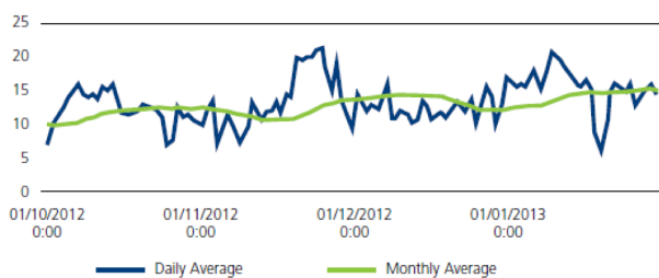
Fig. 30. Percentage of local renewable generation versus overall energy consumption in the area as a result of Smartcity project.
