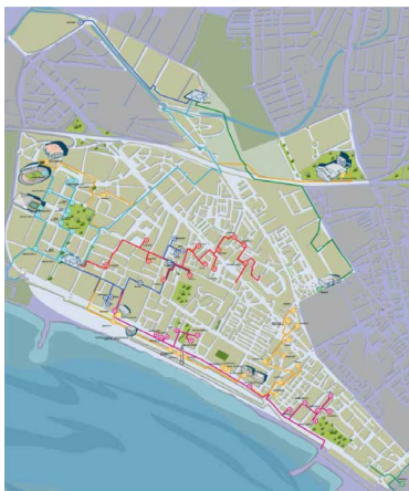
Fig. 23. Geographical scope of Smartcity project in the western coastal area of Málaga. The layout of the five MV feeders and the location of secondary substations are also shown.
