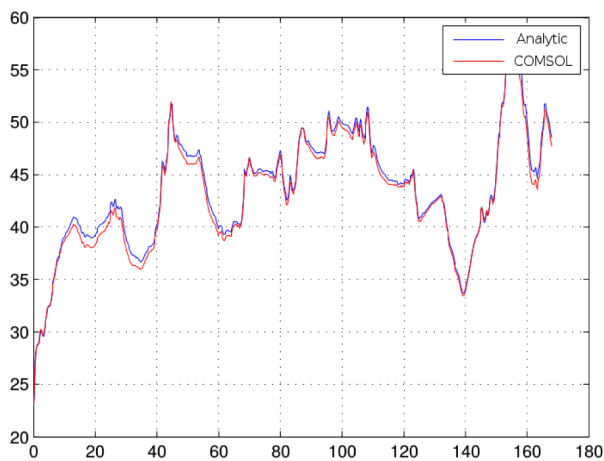
Fig. 17. Comparison of analytic versus FEM simulation (temperature in degrees Celsius and time hours).
