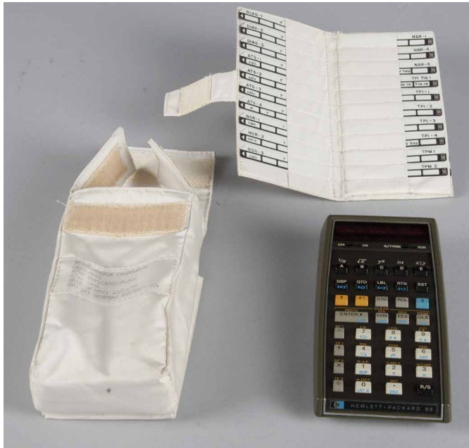
Fig. 3. HP-65 programmable calculator, configured by NASA for use in space. Photo Credit: Smithsonian National Air and Space Museum (TMS A20120307000c07).
