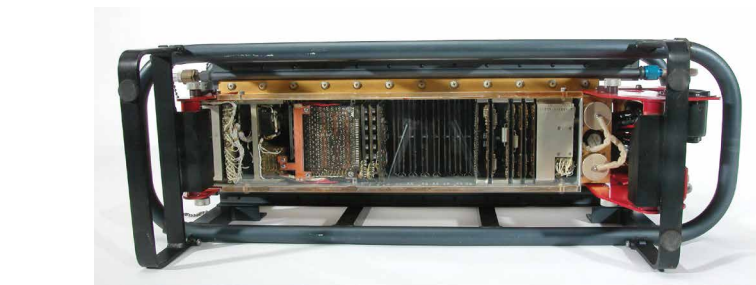
Fig. 2. Lunar Module Abort Electronics Assembly, in its handling fixture. Photo Credit: Smithsonian National Air and Space Museum (TMS A19731554000cp04).
