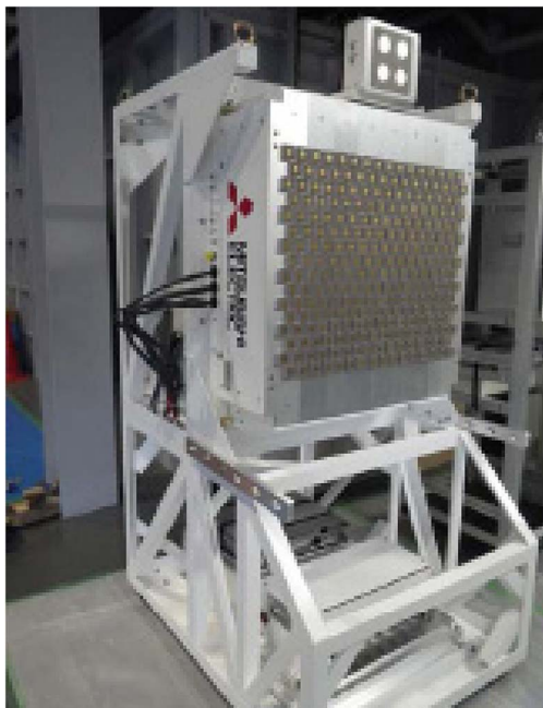
Fig. 22. New phased array for MPT with GaN FET and F-class amplifier circuits installed at Kyoto University and developed by Mitsubishi Electric Corporation in FY2010.
