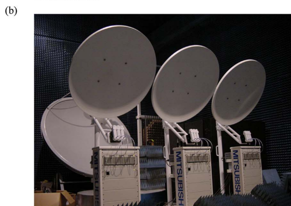
Fig. 14. Parabolic phased array using DDS/PLL oscillators. (a) System block diagram. (b) Image of the array.
