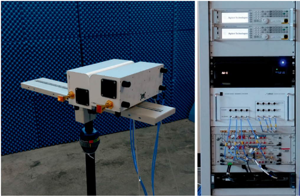
Fig. 8. Apparatus involved in the CREW setup, as shown in [80]. A radar RF module with a single transmitter and receiver is shown on the left-hand side, and the waveform generators, digitizers, and other signal processing equipment mounted on a standard rack are shown on the right-hand side.
