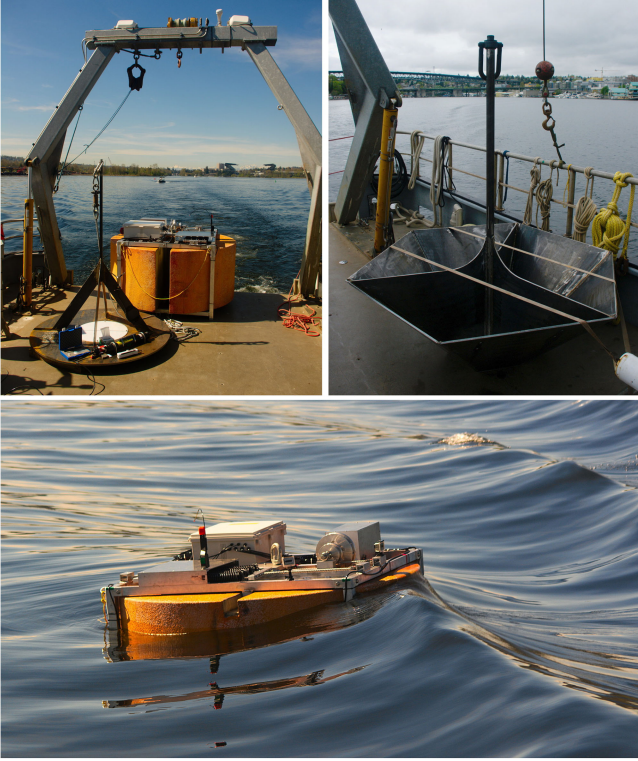
Fig. 5. Left: The miniWEC and flat heave plate on the work deck of the R/V Robertson before deployment. Right: The hexagonal conic heave plate during transit to the test site. Bottom: The miniWEC was deployed on Lake Washington. Due to calm conditions, boat wake was used to excite the surface float.
