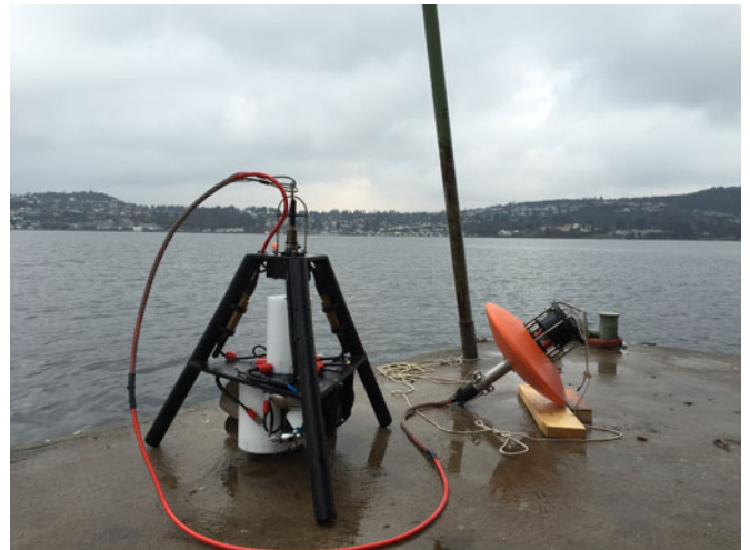
Fig. 1. The NILUS MK 2 bottom node, with the new software-defined modem (transducer in special float shape for stability in currents).
