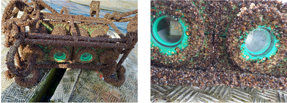
Fig. 11. Condition in August 2021 at the end of the first measurement period. The two middle camera dummies are D4 (left) and D3 (right). The two outer camera dummies were not illuminated in the summer tests to serve as a benchmark.
