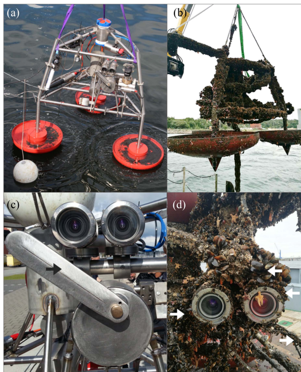
Fig. 2. (a) Deployment of the stationary UFO with clean and untreated surfaces in Kiel Fjord in April 2016 and (b) its retrieval 24 weeks later. The weight difference due to overgrowth by mostly barnacles and mussels was approximately 500 kg given an initial weight of 350 kg, i.e., the mass was more than doubled. Close ups: (c) Stereo-camera of the stationary UFO in frontal view in the clean and untreated status and (d) after its retrieval. The black arrow in (c) indicates the arm of the wiper, which, when in operation brushes over the glass fronts of the two cameras. The white arrows in (d) point to various life stages of the blue mussel Mytilus edulis settling on available UFO-surfaces.
