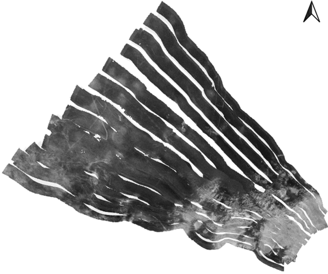
Fig. 3. Backscatter mosaic from multiple survey lines at 100 kHz from Bedford Basin 2016 after noise removal. Note that there are missing areas in the mosaic even though the overlap is close to 50%.
