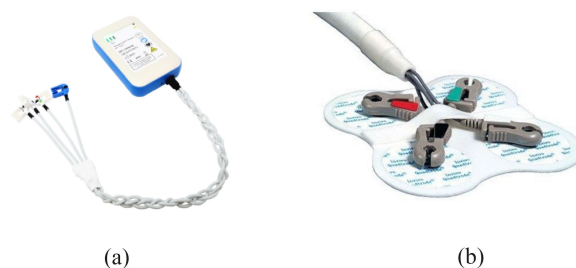
Fig. 10. Example of available ECG-based sensors: (a) Wireless ECG unit for sensing in MR environment [32]. (b) Quadrode ECG electrode for the MR gating [33].
