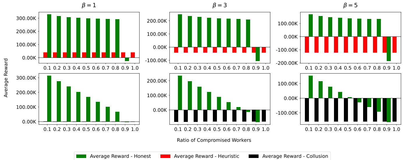
Fig. 7: Average reward with varying ratio of colluding and heuristic workers under different penalty \beta . Federated Learning setting with 10 workers running LeNet on EMNIST digits for 10 epochs. For all experiments, 40000 data points from the MNIST data set were used as public dataset X^{pub} .
