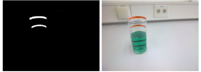
Fig. 4. Binary image of orange pixels (left) and extracted strip components (right).
