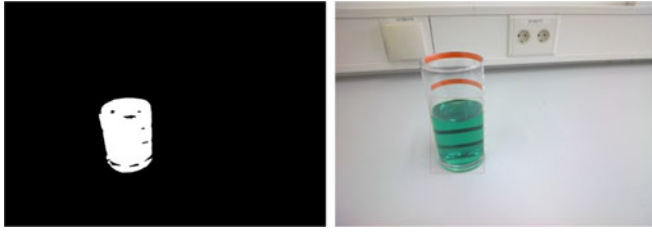
Fig. 3. Binary mask of green pixels (left) and extracted fluid component contour line and bounding rectangle (right).
