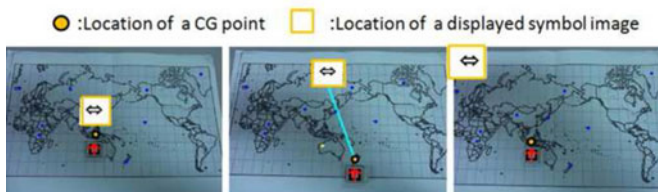
Fig. 6. Three display methods. On the left is AR Annotation wherein a label is placed near the relevant part of the map. The middle and right are control scenarios wherein a label is displayed randomly on the map with a connecting line, and a label is displayed consistently at the top left of the HMD screen without a connecting line, respectively [35].
