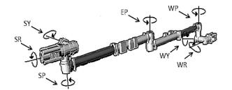
Fig. 2. Three-dimensional representation of Canadarm2 illustrating its seven joints.
