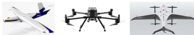
Fig. 5. UAV classification. From left to right are a fixed-wing UAV, multirotor UAV, and hybrid fixed-wing multirotor UAV.
