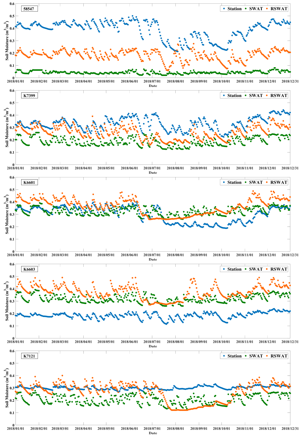
Fig. 3. Simulated SM by SWAT and RSWAT at soil depth of 10 cm against stations.
