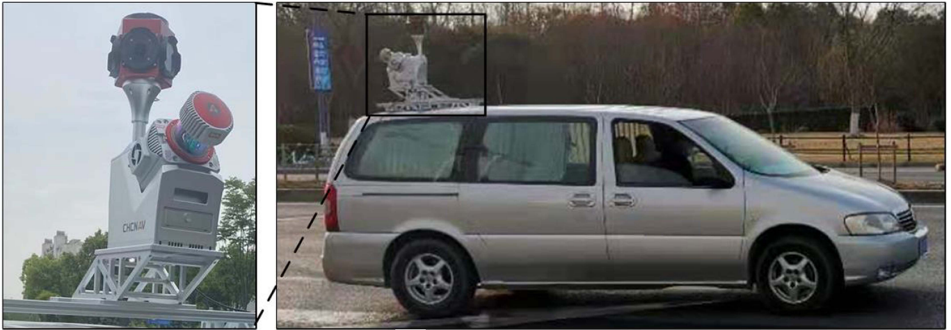
Fig. 12. Mobile laser scanning system.
