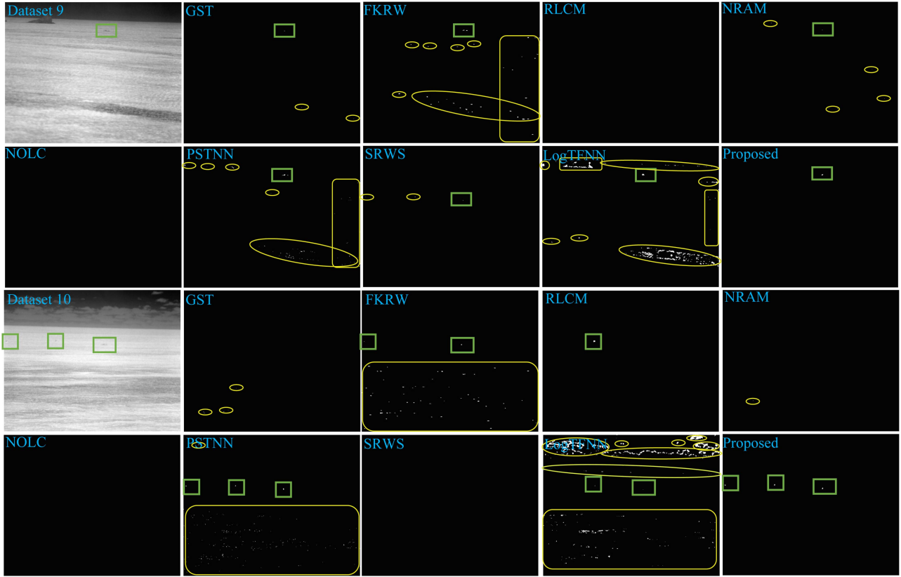
Fig. 11. Qualitative comparison results of Datasets 9–10 between the proposed ICEW method and the baseline methods. The yellow circles indicate false alarms.
