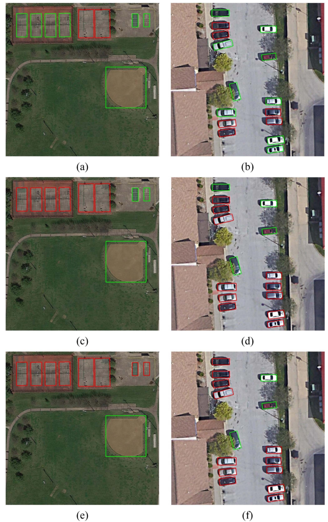
Fig. 5. Dense objects and nondense objects judged by the determination method with different values of moderator a . Objects boxed in red are dense objects and those boxed in green are nondense objects. (a) and (b) Results of the determination of dense and nondense objects at a moderator a of 3. (c) and (d) Determination results at a moderator a of 5. (e) and (f) Determination results at a moderator a of 7.
