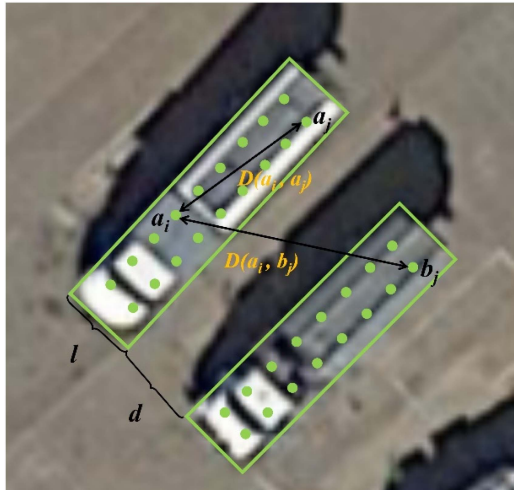
Fig. 3. References in dense object determination method. Green box is the object range. Green dots in the box represent the sample points in the object. D(a_i, a_j) denotes the distance between two sample points in a single object. D(a_i, b_j) denotes the distance between two sample points belonging to different objects. l denotes the minimum side length of the object. And d denotes the minimum distance between two objects.
