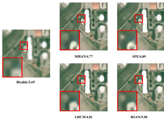
Fig. 7. Visual and image entropy results of real data with a scale factor of \times 8 .
