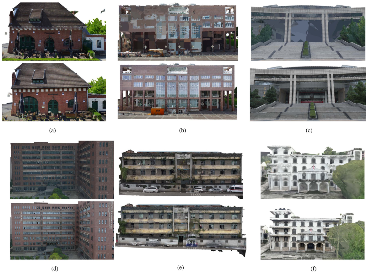
Fig. 10. Qualitative comparison results of texture mesh models on six test datasets. First and second rows show the texture mesh models reconstructed solely from aerial images and the ones fused from both aerial and ground images, respectively. (a) Zeche. (b) Centre. (c) SWJTU-LIB. (d) SWJTU-BLD. (e) CQ-BAISHA. (f) CQ-StudioCity.
