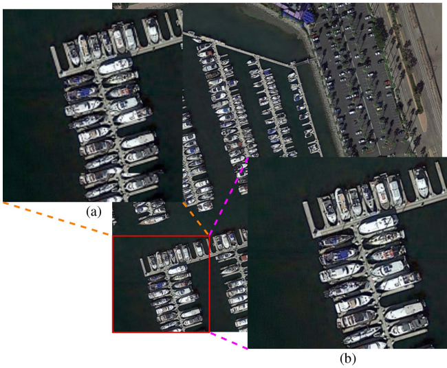
Fig. 1. Diagram of enlarged comparison of the details of objects in the same region between the resolution degraded aerial image and the original HR aerial image. (a) Detailed diagram of the detection object region under the \times 2 resolution degraded image. (b) Detailed diagram of the detection object region under the HR image.
