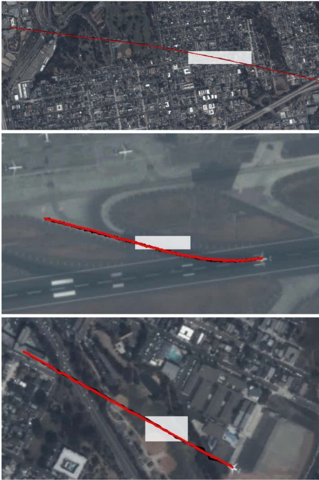
Fig. 14. Tracking performance of our ADMFT on videos occluded by white blocks with transparency 0.8. According to the results, the performance of the ADMFT can remain stable even under a high degree of occlusion.
