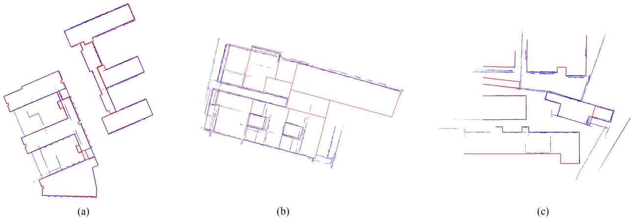
Fig. 17. Coarse registration results. (a) Corner points of Area-A. (b) Corner points of Area-B. (c) Corner points of Area-C.
