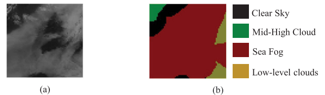
Fig. 2. Cloud image labeled as sea fog with its semantic segmentation mask. (a) Sea fog cloud image. (b) Cloud image corresponds to the semantic segmentation mask image.
