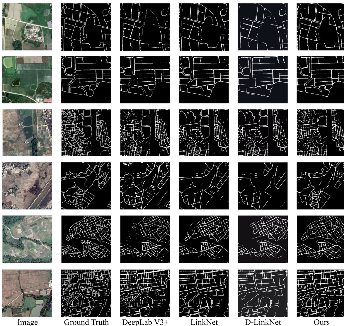
Fig. 6. Visualization of the edge detection results from comparative models.
