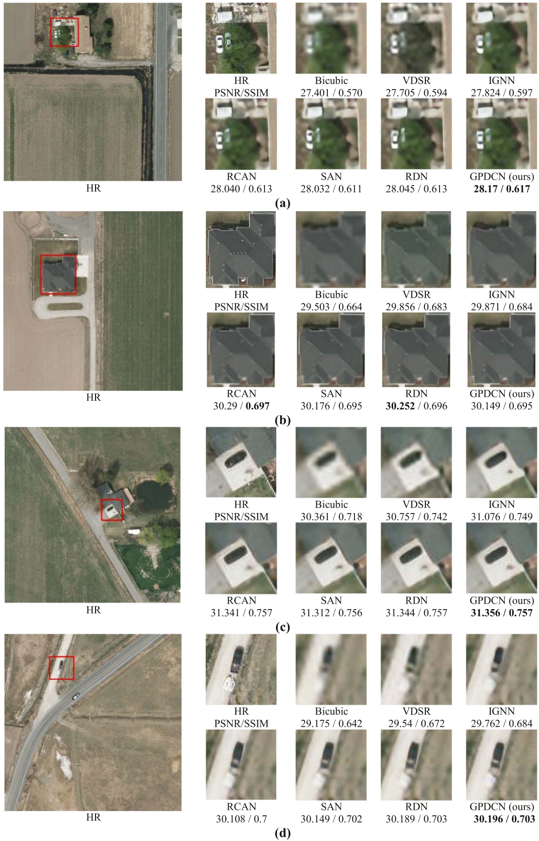
Fig. 7. Reconstruction visual results on 3K VEHICLE_SR and Massachusetts_Roads on a scale of \times 4 for different SR methods. (a)–(d) are from the 3K VEHICLE_SR dataset.
