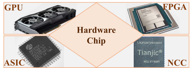
Fig. 32. Four mainstream hardware chips. GPU: Graphics processing unit. ASIC: Application-specific integrated circuit. FPGA: Field programmable gate array. NCC: Neuromorphic computing chip.
