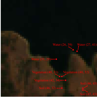
Fig. 17. RGB image of the real Moffett data. The red dots are the visually picked pure pixels.
