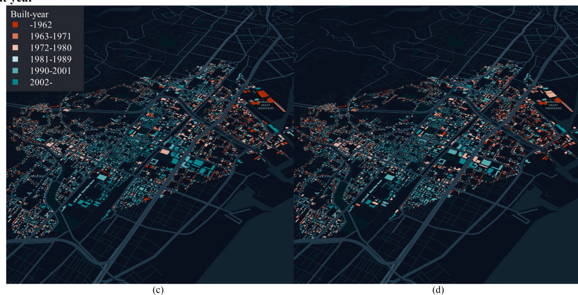
Fig. 13. City-scale predicted building-structure (b) and built-year classification map (d) along with the ground truth (a and c), where different colors represent different building-structure classes. The total number of buildings in this area is 22 392. A total of 6209 buildings are not classified considering that no corresponding SVIs are found or buildings are not located along the road. In addition, the map shows that the spatial distribution of the predicted building structure and built year by the proposed model matches the ground truth. (a) Ground truth. (b) Predicted. (c) Ground truth. (d) Predicted.
