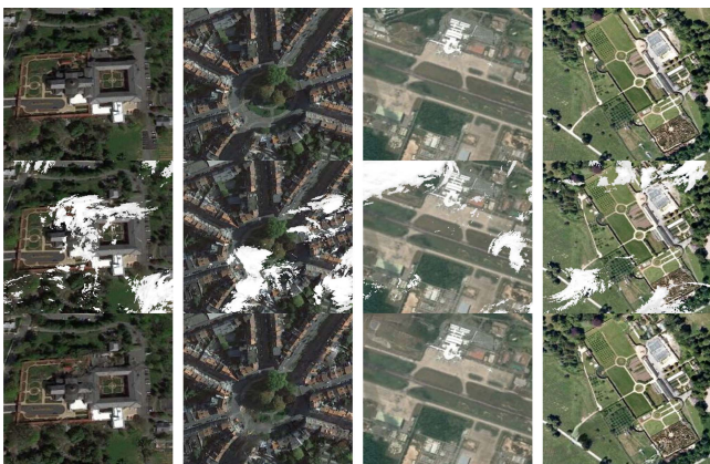
Fig. 11. Thick cloud removal in other complex scenes. The first row is the raw image, the second row is the synthetic cloud image, and the third row is the image after cloud removal.
