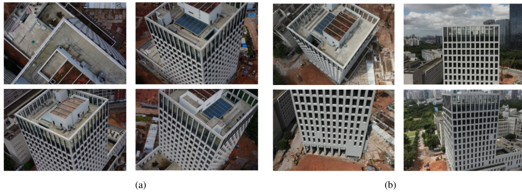
Fig. 14. Illustration of recorded images from oblique and optimized views photogrammetry. (a) Oblique photogrammetry. (b) Optimized views photogrammetry.
