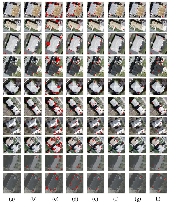
Fig. 9. Some building samples of the Massachusetts Buildings dataset and the building corner extraction results of different corner detectors: (a) original image; (b) ground truth; the building corners of (c) Harris; (d) SUSAN; (e) FAST; (f) CPDA; (g) ECFRNet; and (h) ours.
