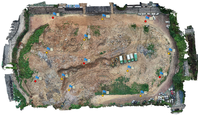
Fig. 5. Experiment site and targets. Red dots represent the control points; yellow dots represent the checkpoints.
