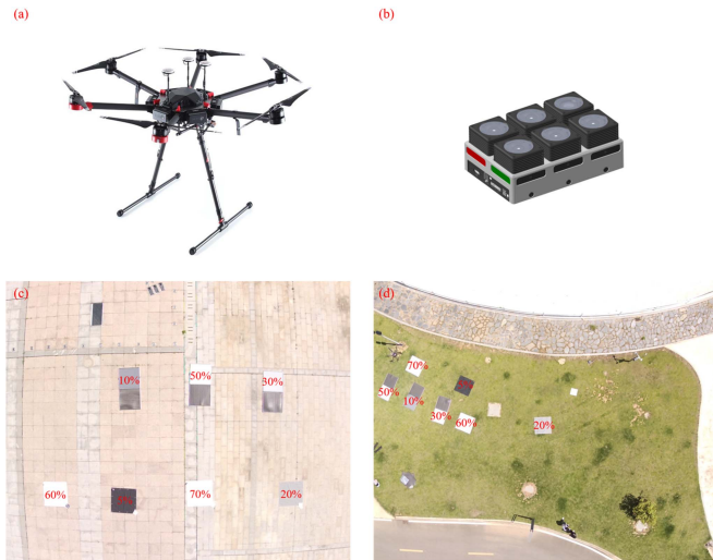
Fig. 2. Distribution of reflective boards in different experimental sites. (a) Unmanned aerial vehicle. (b) Sensor. (c) Brick land. (d) Grassland.
