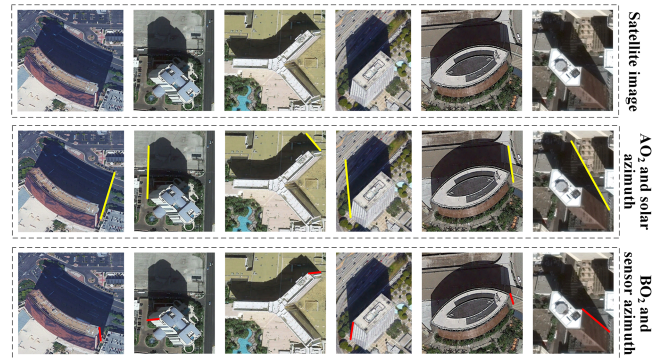
Fig. 9. Illustration of buildings visualized by the VHR image, the line segment for accessing the length of AO_2 and the sensor azimuth ( \theta_1 ), as shown in Fig. 5(c), and the length of BO_2 and the solar azimuth ( \theta_2 ), as shown in Fig. 5(b).
