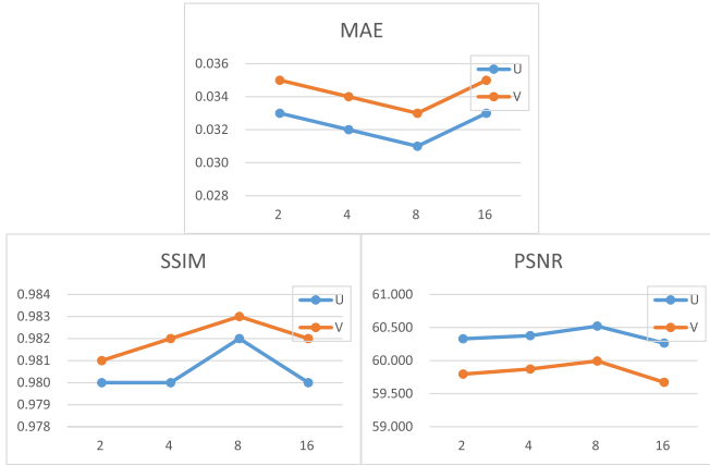
Fig. 9. Sensitivity analysis about the number of denoise blocks.
