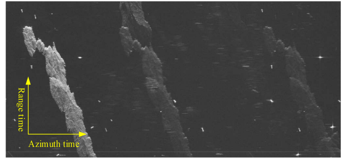
Fig. 15. Imaging results after reconstruction by RD algorithm without channel phase error compensation.
