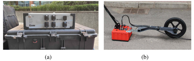
Fig. 13. (a) and (b) Host, antenna, and odometer of the GSSI's SIR-30 GPR.
