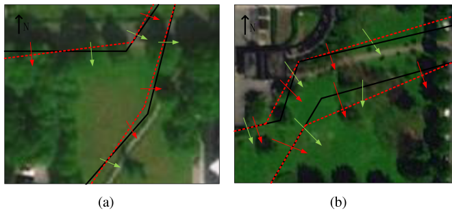
Fig. 14. (a) and (b) Two selected areas, existing and revised pipeline maps. The black lines indicate the pipelines on the existing pipeline map. The green lines with arrows indicate the GPR's detecting direction and position. The red dashed lines are the modified pipelines, and the red arrows indicate some more detections conducted to validate the obtained results.
