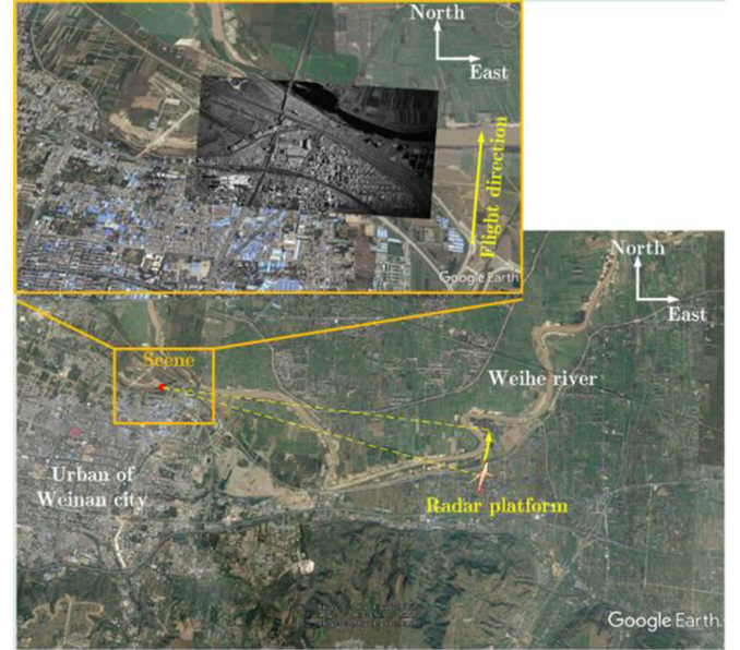
Fig. 5. Observation geometry of radar and illuminated scene, where optics images were from Google Earth on August 13, 2018, and the HH-pol amplitude SAR image, which overlaps on Google Earth optics image, was acquired by the airborne radar system, in April 2017.
