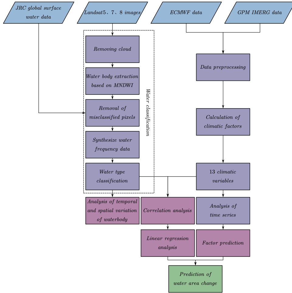
Fig. 3. Flowchart of the analysis of spatial–temporal variation characteristics of the water bodies and their climatic drivers over the Qinghai–Tibet Plateau in 2002–2020.
