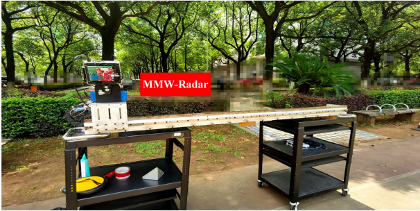
Fig. 16. 77-GHz millimeter-wave SAR system for the real measured experiment. The electric rail length equals 1.57 m and the radar height equals 1.40 m.
