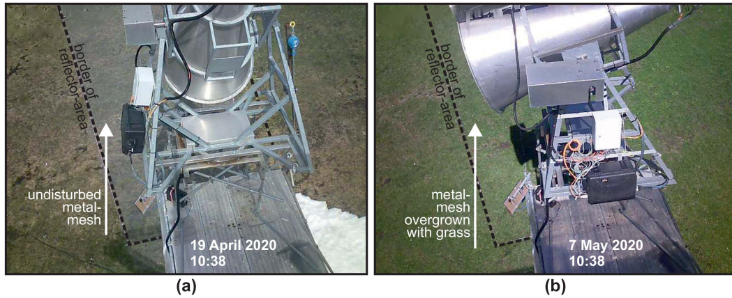
Fig. 7. Pictures from the instrument surveillance camera on (a) 19 April 2020 10:38 CET after the snow melt, and (b) 7 May 2020 10:38 CET near the end of the Campaign C4. The vegetation growth is evident in panel (b).
