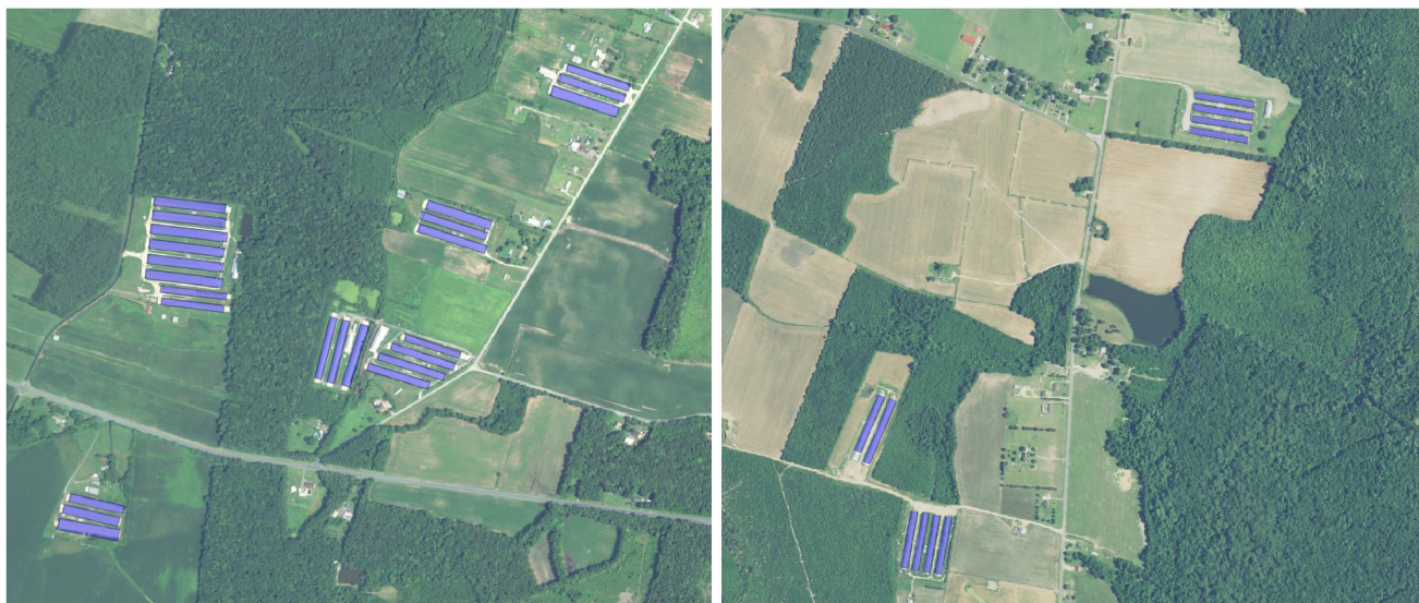
Fig. 7. Example model predictions (highlighted in blue) from two counties that the CoA reports zero poultry operations in. (Left) Twenty-four predicted poultry barns with NAIP 2017 imagery over a 2.6-km 2 area from Sussex County, Delaware. (Right) Ten predicted poultry barns with NAIP 2016 imagery over a 3.1-km 2 area from Robeson County, North Carolina.
