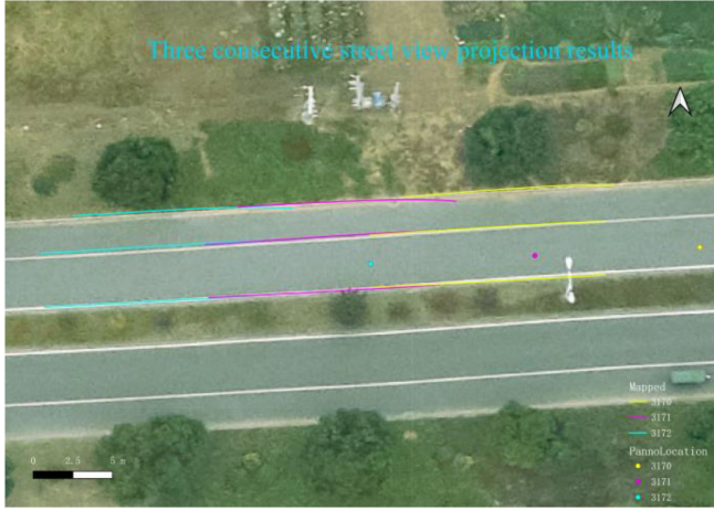
Fig. 10. Projection results of longitudinal markings for three consecutive street-view images.
